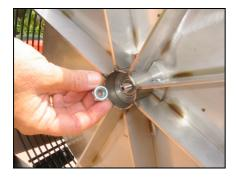
Take the flywheel and remove the plastic dust protection cap from the hub.
