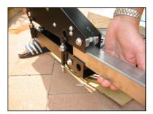
Now slide the main frame assembly onto the main bar with the shaft side pointing away from the seat.
