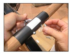
Pull the chain out approx. 60 centimetres. Put a clothes peg onto the chain close to the main bearing block to prevent it from recoiling. Take the 6 mm U-bolt and put it through the slot in the chain-handle connector.
