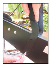
2 'boomerang' metal plates are included with the machine - serving as a chain guide attached to the flywheel cage.
