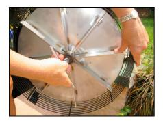
After tightening the tension on the main shaft due to this M10 nut subsequently has to be released. To release this tension, hold the flywheel by the vanes to keep it from rotating, and un-tighten the M10 nut by turning it counterclockwise over approximately 5 degrees (about 1/10th of the distance between two subsequent vanes).
