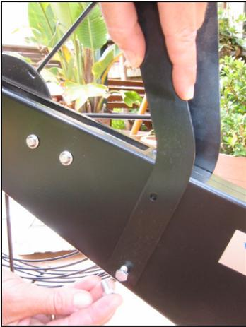
2 'boomerang' metal plates are included with the machine - **servicing as a** chain guide attached to the flywheel cage.
