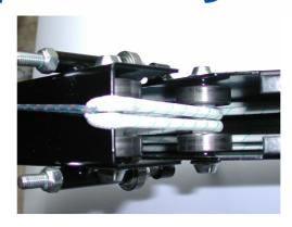
Check whether both ends of the elastic cord have stayed at their proper side; if this is not the case correct it. Take the chain and traveling pulley, stretch the chain and insert the traveling pulley between the two sides of the main frame close to the bottom part. Insert the traveling pulley between the two sides of the elastic cord, and hook the elastic axle with its Starlock washers behind the elastic cord. (El13,El14)
