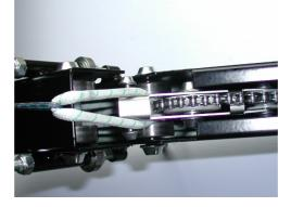
Pull the chain out to take up any slack, and make sure the chain runs correctly over the middle of the chain wheel. Loosen the string cautiously from the hindmost adjustment bolts and release tension slowly. When the chain has reached its final position, and still runs over the chain wheel correctly, pull the string out slowly by one of its ends.(El15,El16,El17)
