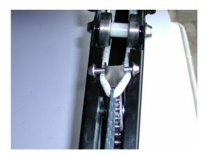
Let the elastic cord recoil completely, pulling the string around the rear axle. Loosen the elastic cord from the rear axles. Keeping the string in position remove the elastic cord. (El2)
