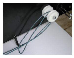
Take the chain and the traveling pulley; move the traveling pulley in between the lower part of the main frame and the upper part to outside the main frame, and fold the chain over to the front. (El3,El4)
