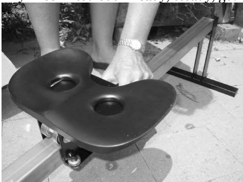
Fix rear leg to 'bent' end of bar, slide on seat from other end.
