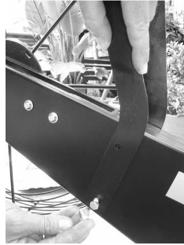
Fit plate to other side using 2 shorter bolts
