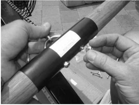
Bolt handle to curved piece, washers inside recessed holes, tighten
