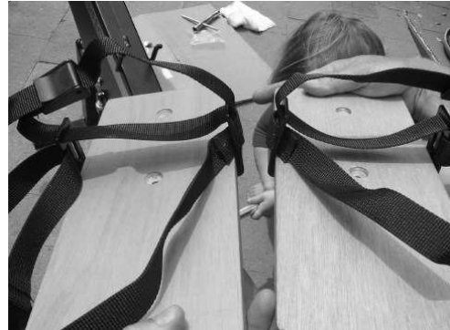
Ensure footstretcher on correct sides; angled plate on inside, against bar
