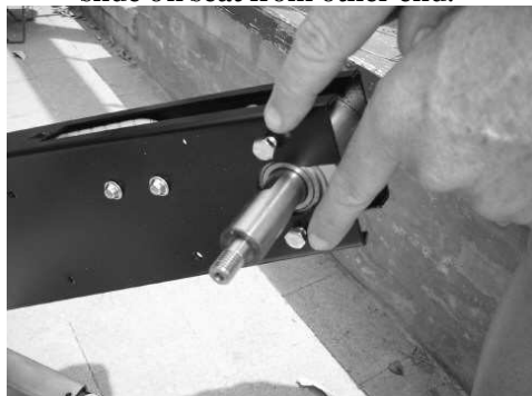
Remove both hand tightened nuts at main shaft
