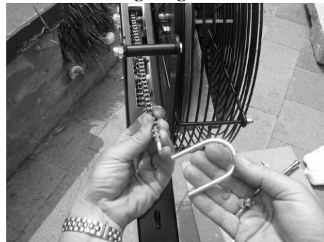
Pull out chain and slide on handle bolt through keyhole piece
