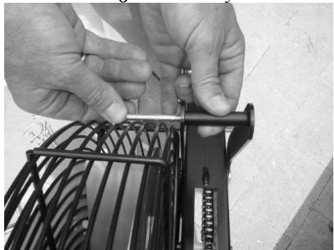
Fit spacer bar & roller to guide plates
