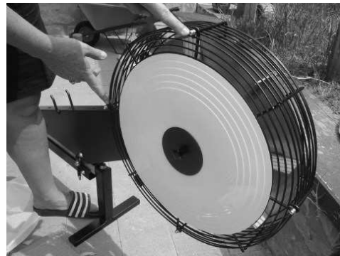
Fit cage cover, fix with 4 capped nuts Finger tighten
