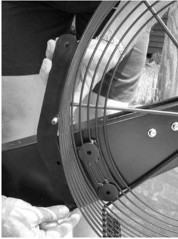
Guide plate fits between cage & main housing, using 2 longer bolts
