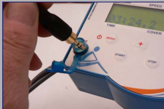
The microphone connector is a waterproof jack, with a sealing cap.
